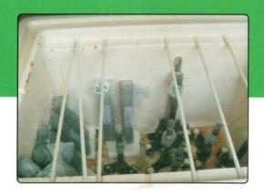
Intergranular Corrosion Testing is carried out as per ASTM A262 for austenitic stainless steels.
